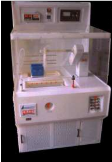
Semi Automated Twin Bath BOE Station
