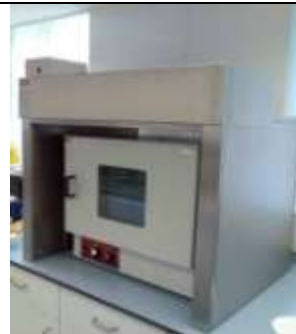
Oven Extraction Hood for Odour Extraction with optional Carbon Filtration
